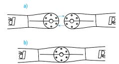
Insert the six propeller bolts into the propeller plate. Align the bolts with the mounting holes and insert into the propeller.
