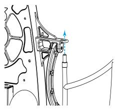
Insert the nylon connector, located at the end of each leg, into the cage section. Push the cage section until the location pin engages and secures the cage section in position.
