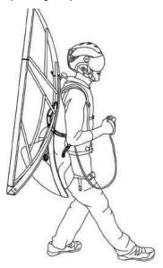
The turning propeller can cause considerable damage and injury. Be aware and keep persons at a safe distance. After prolonged engine use stay clear of hot engine parts and exhaust muffler.
