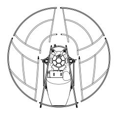
Starting with a lower cage section, insert the cage dowel into the mounting aperture located on the hinge block, making sure the cage section is curved towards the rear of the paramotor.
